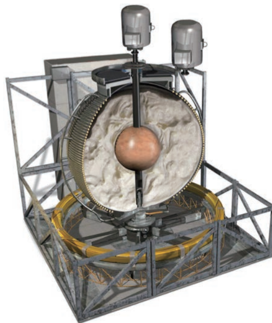
Rendering of the 3 m experiment. The inner sphere and the outer spherical shell can be driven independently by their two respective motors ( top ). Liquid sodium serves as the working fluid for hydromagnetic experiments
